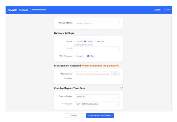
Click Create Network & Connect. The device will deliver the initialization and check the network connectivity.
