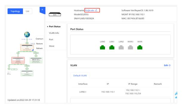
• Click **List** in the upper-left corner of the topology to switch to the device list view. Then, you can view device information in the current networking. Click an item in the list to configure and manage the device separately.
